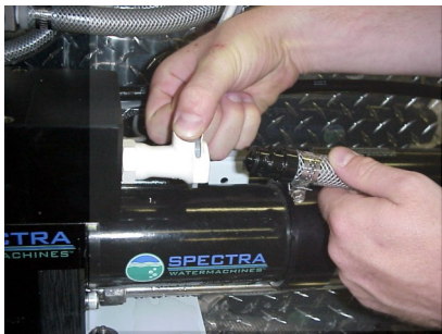
Connecting brine discharge service hose
