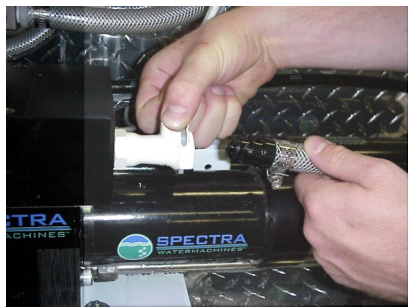
Connecting brine discharge service hose
