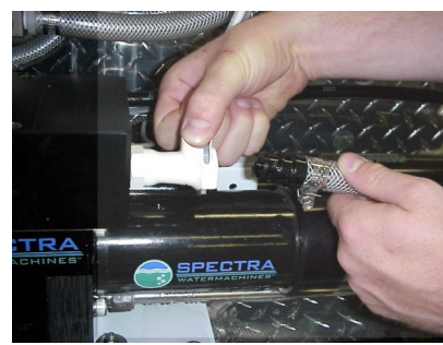
Connecting brine discharge service hose
