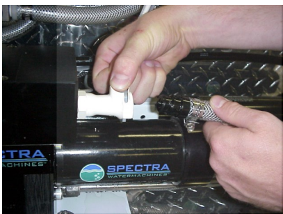
Connecting brine discharge service hose
