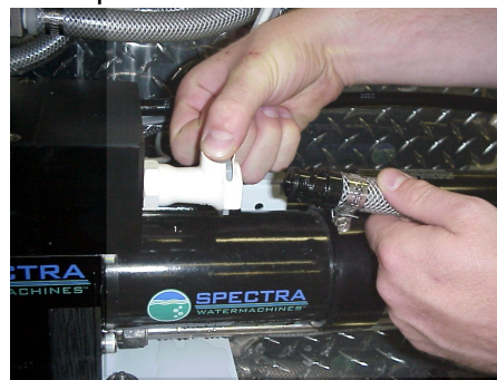
Connecting brine discharge service-hose
